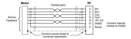
Figure 20 - SinCos cable connections
